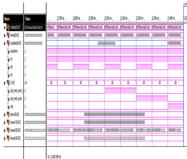
Figure. 5.1(b) Simulation results for direct key
