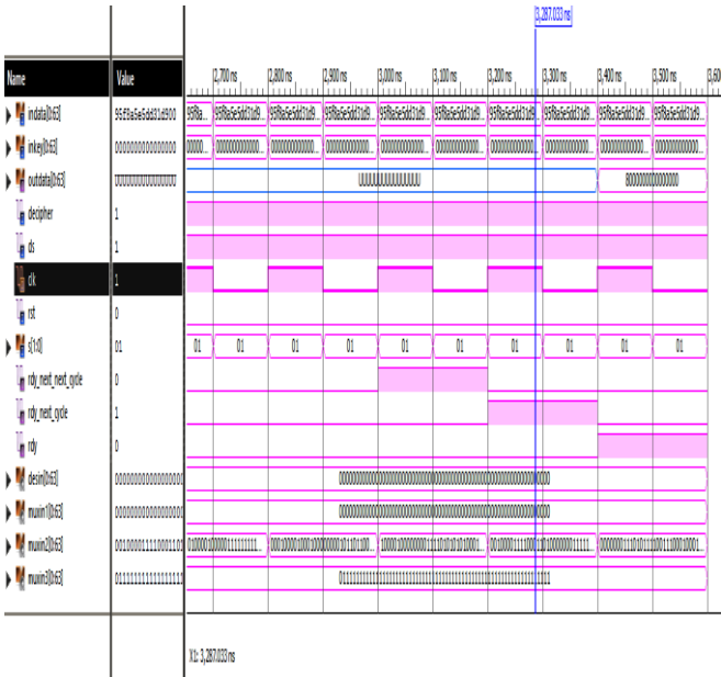
Figure. 5.2 (b) Simulation results for key generated by LFSR
