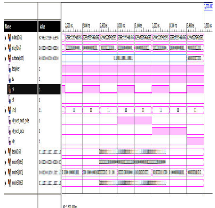
Fig. 5.4(b) Simulation results for key generated by 2's complement.
