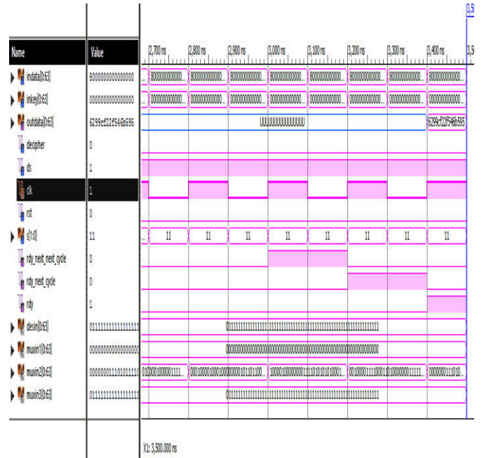
Fig. 5.4(a) Simulation results for key generated by 2's complement.
