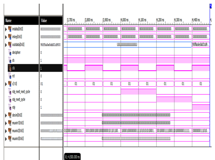
Figure. 5.2 (a) Simulation results for key generated by LFSR
